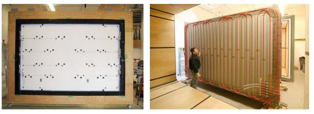
In all cases the insulation materials were installed between the studs to achieve a nominal insulation R-value of 13 (when measured in accordance with FTC Title 16 CFR Part 460).
